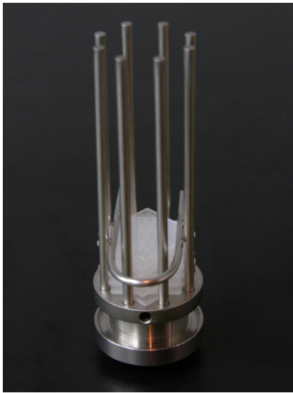
Place coated chip back and then put in the removal tool.
