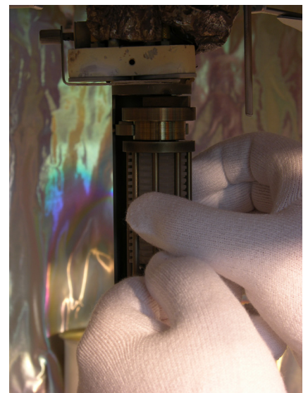
Lift chip stack and lift magazine, then pull straight out.
